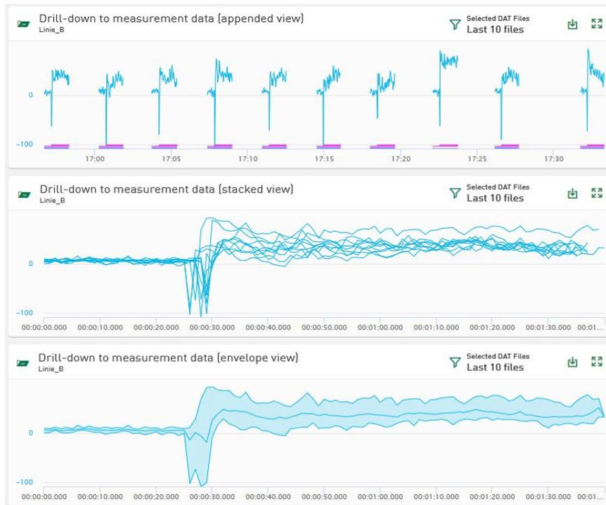
Several measurement files can be appended to each other (top) or compared directly in the stacked view (middle). In the envelope view (bottom), the maximum, mean and minimum values are displayed as trends.
